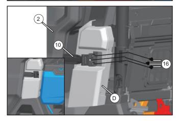
Align the LH lower connecting plate assy (10) on the LH rear half door (2) with the corresponding holes on the vehicle and install three M8x16 inner hex screws (16), re-assemble the left side panel, rear seat (D) then reset the rear cargo. 🕞 СFМОТО
