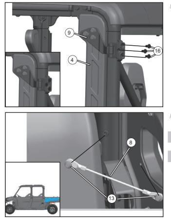
Align the LH rear upper hinge assy (9) on the LH front adapter bracket (4) with the corresponding holes on the vehicle and install three M8x16 inner hex screws (16).
