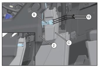
Align the LH lower connecting plate assy (9) on the LH front half door (2) with the corresponding holes on the vehicle and install three M8x16 inner hex screws (15), then reinstall the left side panel, front seat (C).
