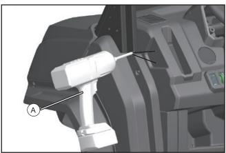
Drill two 9mm holes through the plastic at the reserved marks of the vehicle with an electric drill (A).
