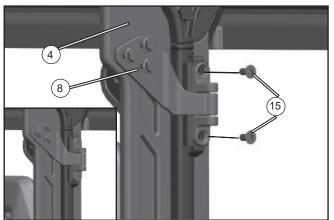
Align the LH rear upper hinge assy (8) on the LH front adapter bracket (4) with the corresponding holes on the vehicle and install two M8x16 inner hex screws (15).
