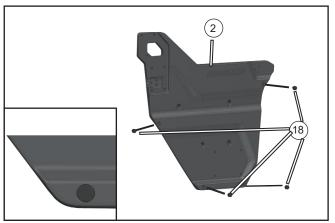
// Install four rubber mats (18) into the corresponding holes of the LH half door (2) at the locations shown.
