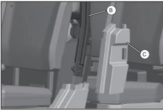
Remove the left side panel, front seat (C) from the cab frame (B).
