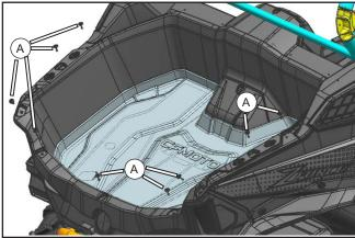
Remove the M6x20 screws (A) from the top edge of the rear cargo box.
