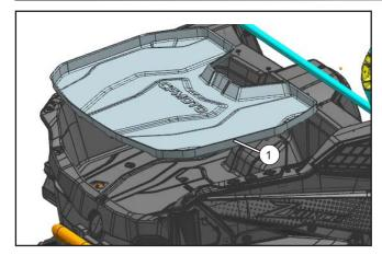
Set the cargo mat (1) into the cargo box at the rear of the vehicle.
