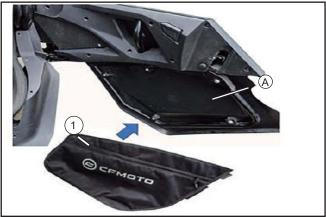
// Put the storage bag, LH side door (1) at the preassembly position of the LH side door (A).
