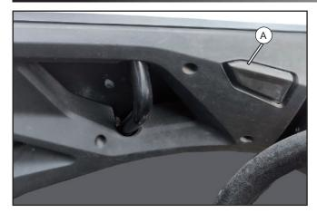
// Press the door lock (A) to open the LH side door.
