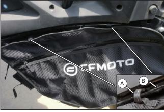
Install the plastic buckles (A) of the LH side door soft bag onto the pipe (B).
