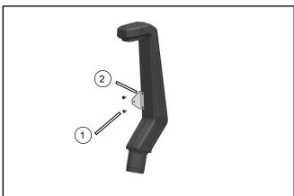
$/\!\!/$  Secure the center bracket @ at the center position of the air intake schnorkel with bolts @ .
