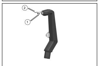
${/\!/}$  Secure the top bracket  ${@}$  on the top position of the air intake schnorkel with bolts  ${@}$  .
