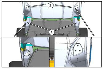
Use hole saw to open holes at the rear bed side panels
