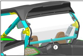
// Tilt the windshield assembly (2) and position it between the top roof and the top bar front assembly.
