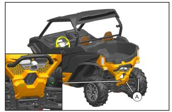
Remove the oringinal screw (A) as shown.
