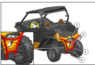
Place the rear bumper (2) at the assembly position. Install the bolts (3) at upper position and bolts (5) at the lower position, then tighten them sufficiently. Install the deco plug (4) onto the head of bolt (3).
