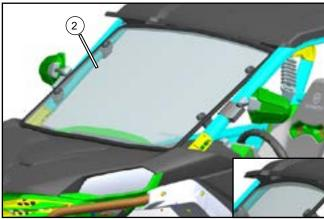
Tilt the windshield assembly (2) and position it between the top roof and the top bar assembly.
