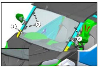
Determine the clamp positions, then secure clamps (3) on each side as shown. Hand-tighten the clamp screws sufficiently, using care not to over-tighten.
