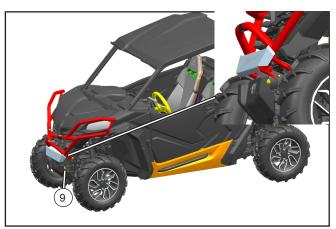
// Install the deco cover assy on the front of the bumper with bolts (9).
