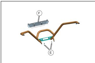
Remove the bolts (E), and deco cover (F). Save the bolts and deco cover for reinstallation.
