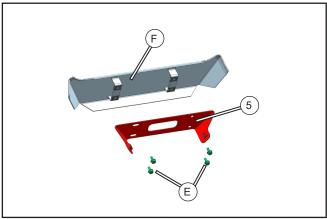
// Install the deco cover (F) on deco plate bracket (5) with bolts (E).
