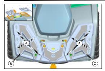
// Unscrew the screws (A), then remove the covers (B,C).
