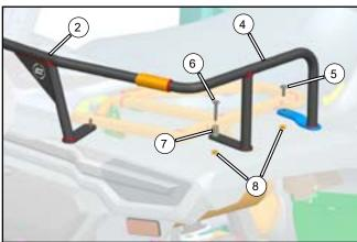
Put the bushing (7) in the right position shown in the picture, secure the right nerf bars (4) with screws (5,6) and self lock nuts (8). Do not fully tighten at this time.
