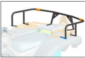
// Tighten all screws (5,6) and self lock nuts (8) with allen wrench and open-ended wrench.
