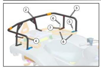
The installation method of left nerf bars (3) is the same as that of right nerf bars (4).
