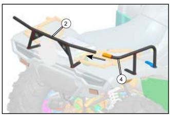
// As shown in the picture, connect the right nerf bars (4) with the middle nerf bars (2).
