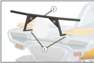
Install the middle nerf bars (2) with screws (5). Do not fully tighten at this time.
