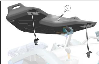
Align the rear locking grooves of plastic basket (2) over the installed CF Connect Clamps and set it into place.
