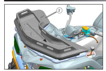
Push the plastic basket (2) along the direction shown in the image to lock the basket to the rear clamps.
