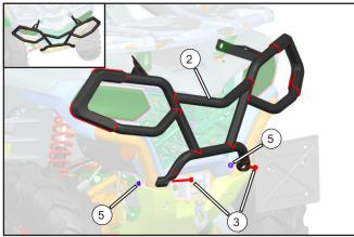
// Tilt the front bumper (2) to a proper position and secure it to the front bracket with bolts (3) and nuts (5) on both sides of the bottom. Do not fully tighten at this time.
