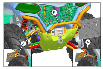
// Unscrew the bolts (A) and remove the original front bumper (B).
