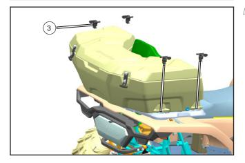
Install the CF connect clamp (3) at corresponding positions, and turn them anti-clockwise to lock them.
