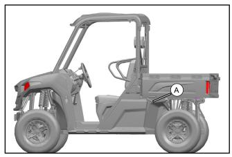
// Open the cargo box by pulling the handle (A).
