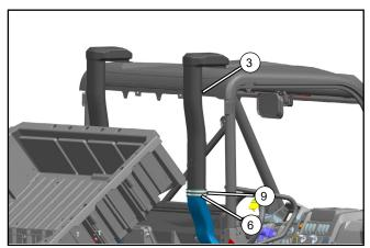
// Install connecting pipe (3) to the air filter inlet using connector (9), and secure with clamps (6).
