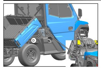
Open the passenger side cover plate and remove the primary filter box (D) attached the air filter housing. Retain the connecting components.
