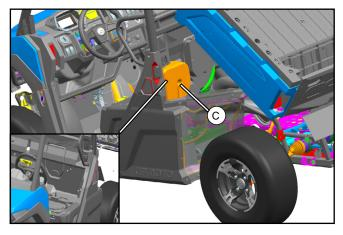
Open the driver side cover plate and remove the CVT inlet box (C). Retain the connecting components.
