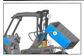
// Install connecting pipe (3) to the CVT air inlet using connector (9), and secure with clamps (6).
