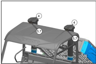
Secure the connecting pipes (3) to the top roof with connecting plates (4), screws (7) and nuts (5).
