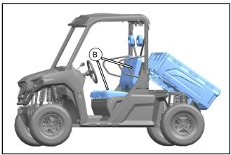
Remove the driver and passenger seat back assemblies (B).
