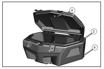
Install the plug (4) at the drain outlet of the rear cargo box (2), and place the spare plug at the position of the upper box cover.
