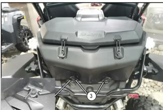
Install two CF connect clamps (3) in the two holes at the rear of the rear rack cover, then secure the cargo box by rotating the levers counter-clockwise.
