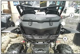
Position the rear cargo box (2) on the rear rack cover (A).
