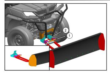
// Insert snow plow assembly (1) into the slots of the snow plow bracket (2).
