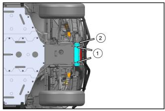
Loosen front skid plate bolts (1) at the location shown. Align the snow plow bracket slots and push the bracket (2) onto the bolts. Tighten bolts (1).
