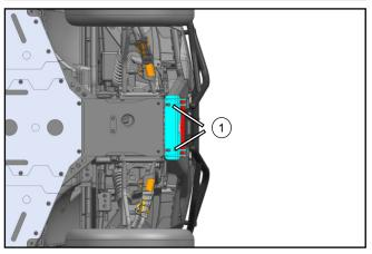
// Tighten bolts (1) at the front skid plate.
