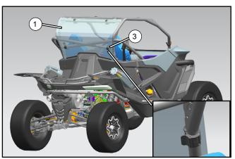
Position the rear windshield assembly (1) on the top bar rear assembly as shown to determine the clamp positions, then assemble each side with clamps 42 (3). Tighten the screws sufficiently, using care not to overtighten.
