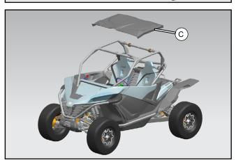
// Remove the top roof (C).
