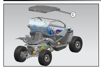
Reinstall the top roof (C).
