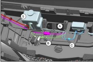
Set up Harness and Washer Tube (5) as the left illustration, Pass switch cable (A) through the front fender and the switch mounting hole, and plug Connector (B) and (C) with Washer Tank cable port and Main Cable port.
