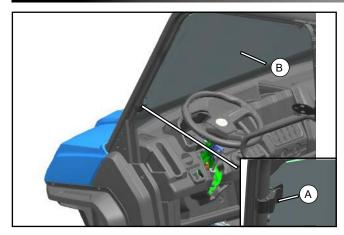
Loose 2 clamps (A) of front Glass windshield, Remove 2 brackets located at the top with thumb screws. Remove front windshield (B).
