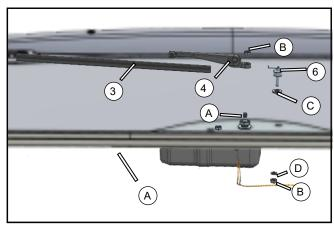
Install Wiper Blade (3) on Wiper Arm (4), and tighten wiper on Wiper Motor with M8 Nut (B). Install Washer Tube Adapter (6) on front windshield with Rubber O-Ring (C), Washer (D), M8 Nut (B). Connect washer tube of Wiper Arm to washer tube adapter.
