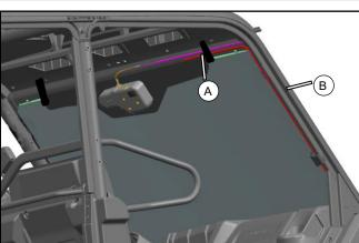
Set up Washer Tube (A) through along ROPS as the illustration, use 3M double faced adhesive tape to stick wash tube, connect the tube with the adapter.
