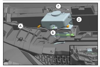
// Insert M6 Nut Clamp (7) into the slot of Front Fender (A), use M6x16 Bolt (8) to tighten Washer Tank (2) on Front Fender as the left illustration.
