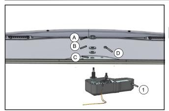
// Install Wiper Motor's M16 Nut (A), Cap Washer (B), Rubber O-Ring (C) and M8 Bolt (D) as the illustration.
