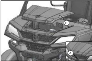
$\ensuremath{/\!/}$  Take out the insert of front hood from (A) place, Remove front hood (B)
