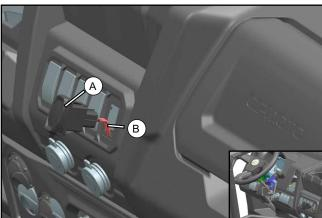
// Connect the Connector (B) of switch cable with switch (A).
