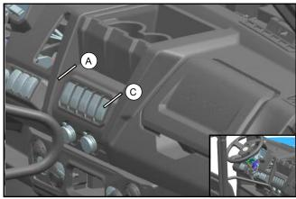
// Use a cutter to cut Switch Mount (C) for installing the switch of Wiper And Washer Assy.
