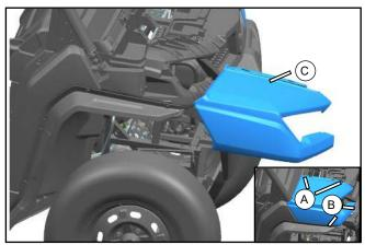
Dis-assemble 2 units M6x12 Bolt (A) and 4 Expansion Screws (B), and Remove Panel (C).
