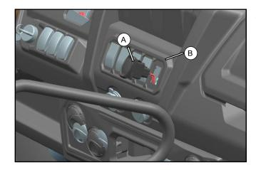
// Install Switch (A) on Switch Mount (B) correctly.
